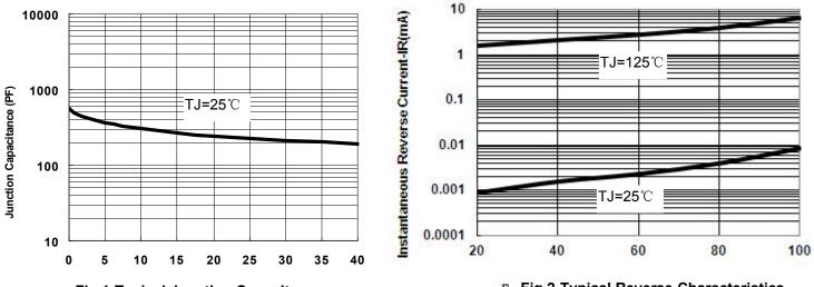
Fig.1-Typical Junction Capacitance
