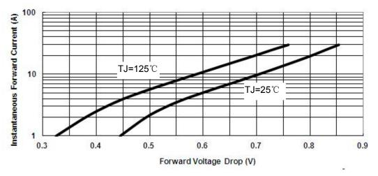
Fig.3-Typical Instantaneous Forward Voltage Characteristics
